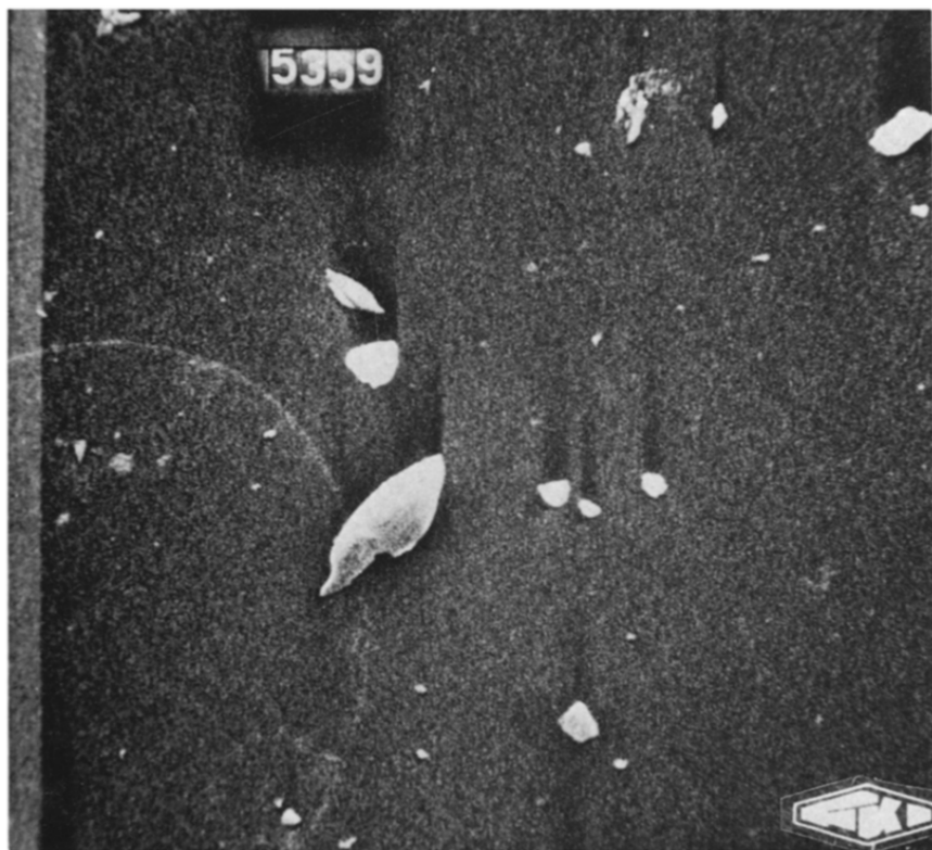
Fig. 3. Scanning-electron microscopic photograph of the glass-lined stainless-steel tubing (magnification \times 1000 ).
